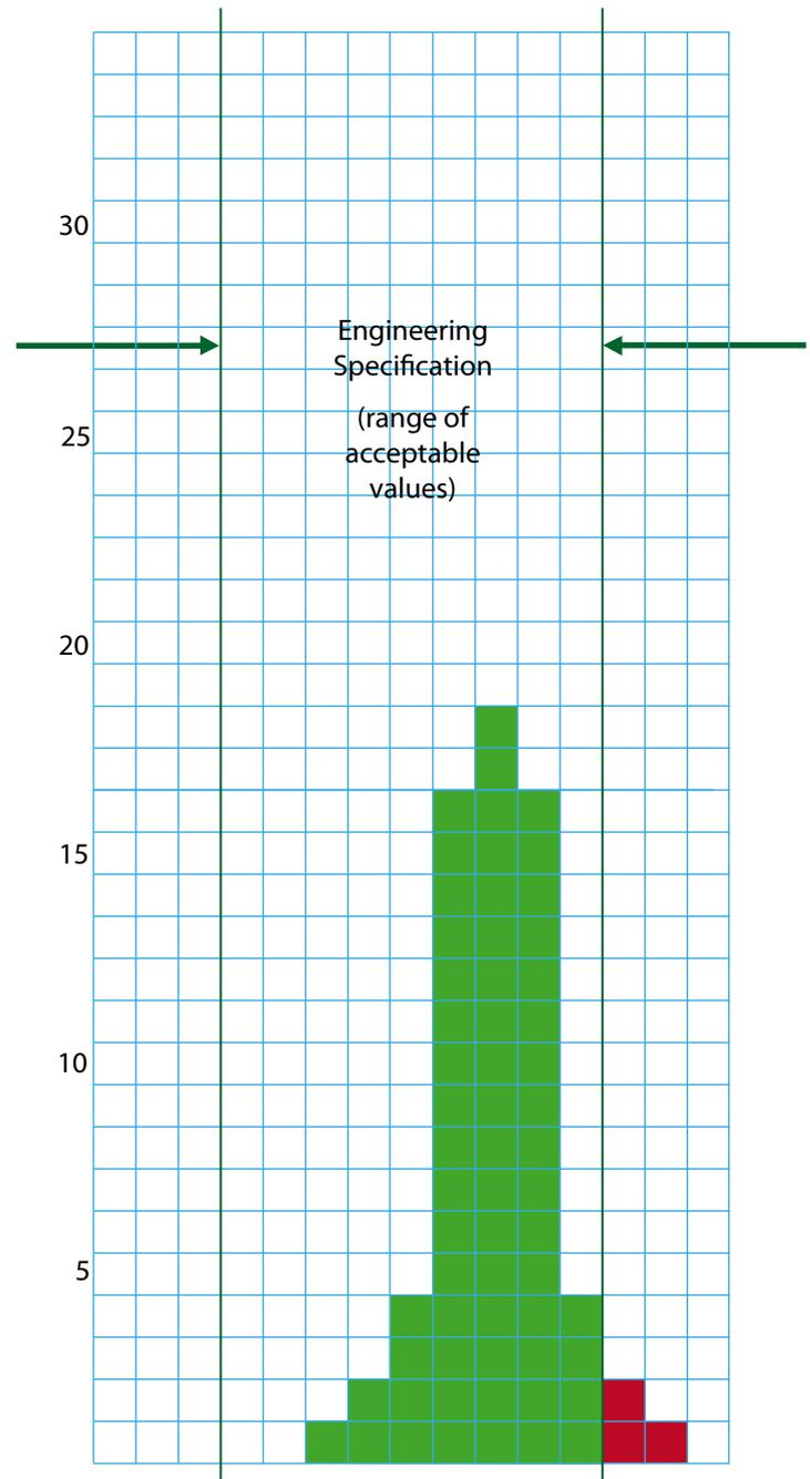
**Figure 2.4** The same degree of variation as in Figure 2.3 but with a shift or drift in the mean value. Defective items produced.
