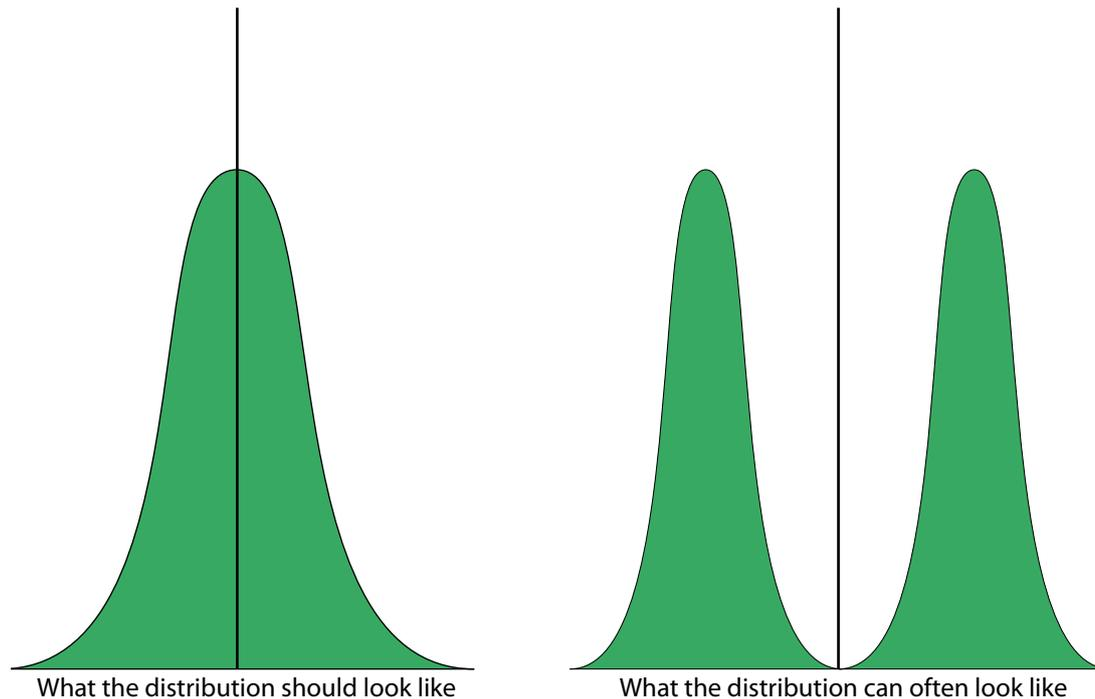
**Figure 2.6** The double humped distribution curve, caused by selecting closer tolerance devices from a large batch in order to offer a choice (e.g. 2%, 5% and 10%) with premium prices for the better devices. This can also occur when devices are selected for shipment to favoured customers.
