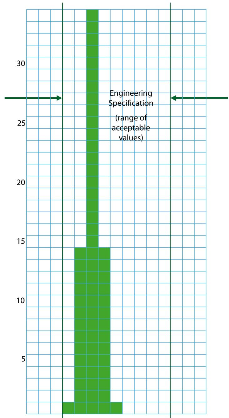
**Figure 2.5** Less variation. Still no defects even though there is a shift or a drift away from the mean value. Beyond Zero Defects!
