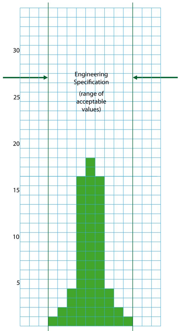
**Figure 2.3** 'Zero defects'—when all items produced are within the engineering specifications—less variation.
