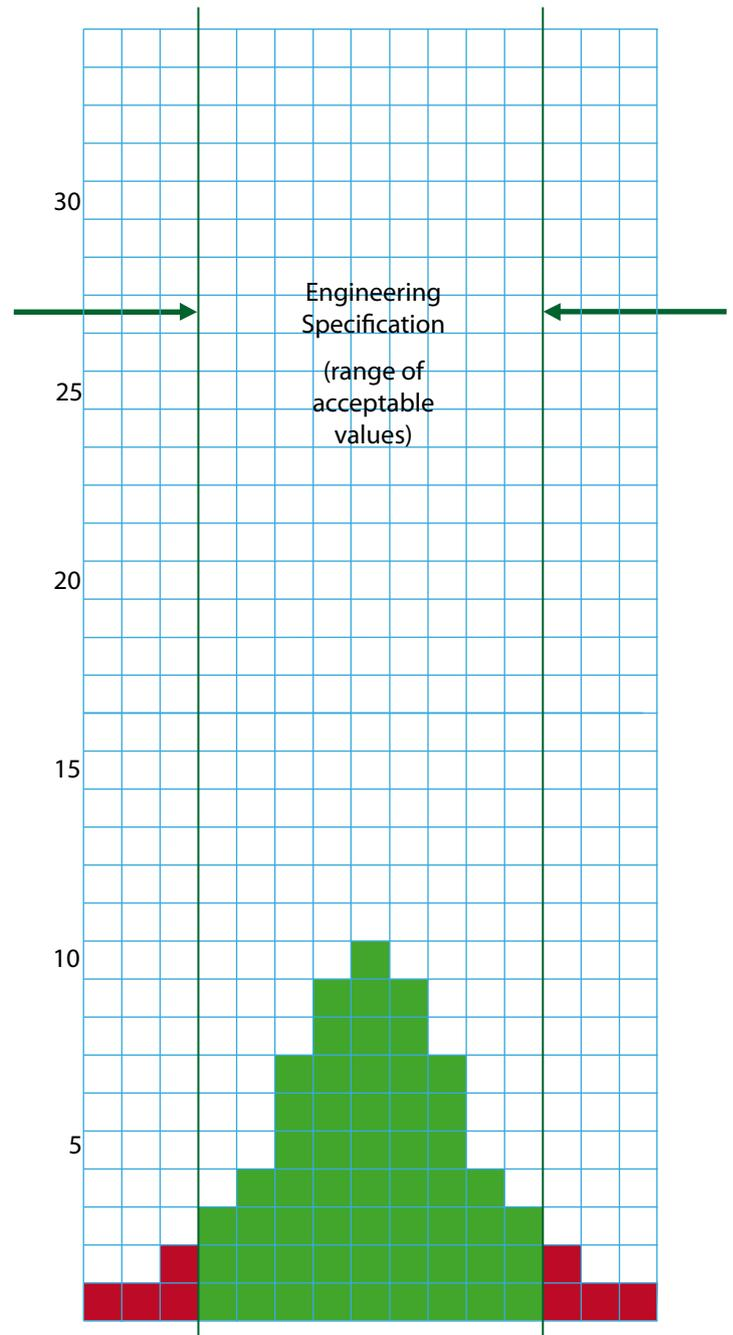
**Figure 2.2** A process that cannot match the engineering specification—too much variation!
